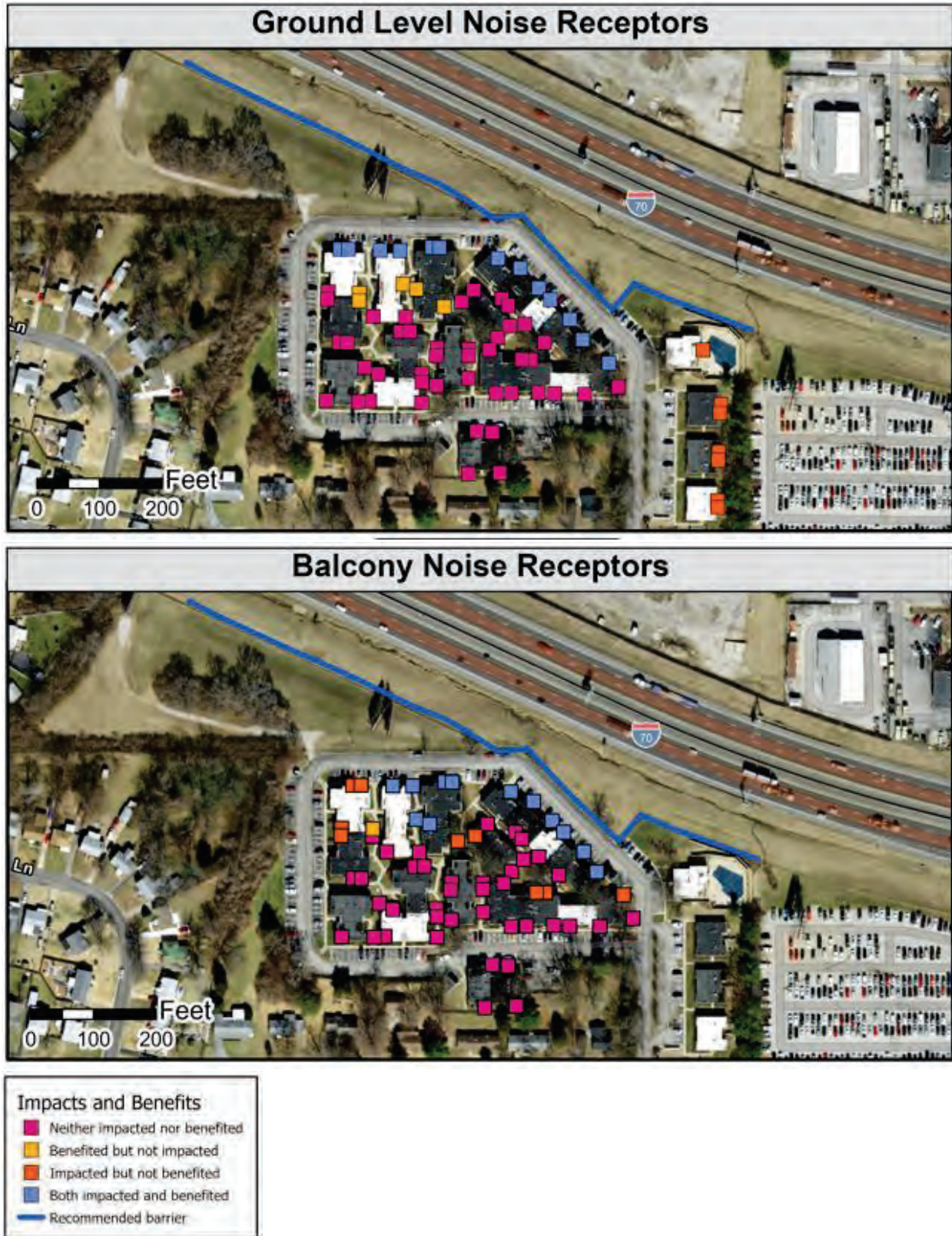
Figure 4.8-7: Recommended Barrier Insertion Results
