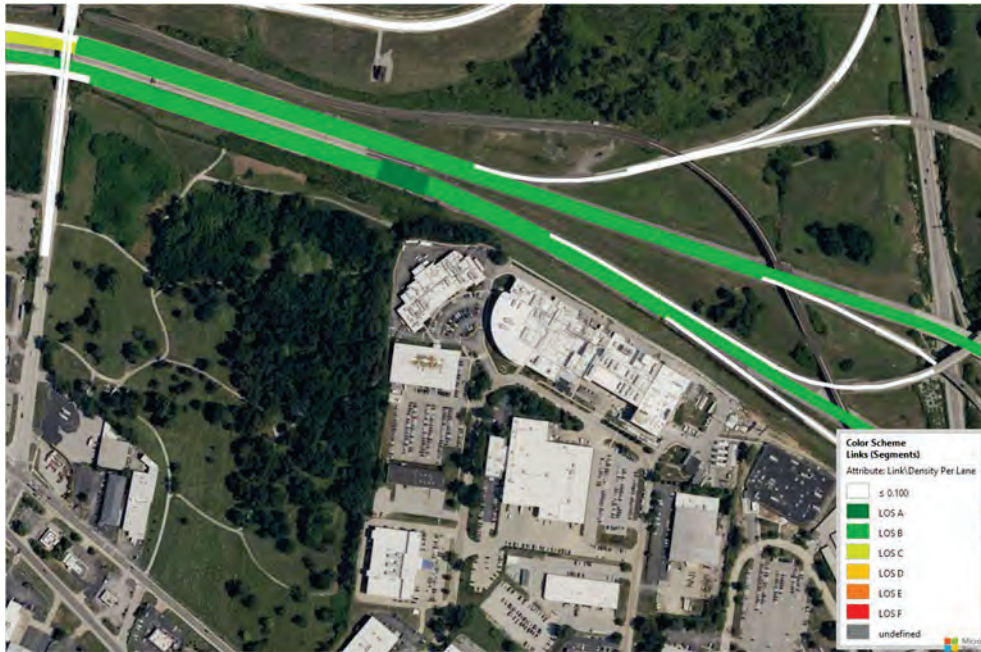
Figure 8 – I-70 & I-170 Weave Level of Service, PM 2037 No Build
