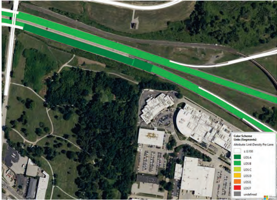
Figure 6 – I-70 & I-170 Weave Level of Service, AM 2037 No Build
